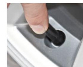
Inspect whether there is any damage or crack caused by installation on the valve surface.
