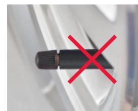
The valve stem should not extend out the rim flange.
