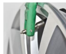
Use a suitable valve mounting tool. Do not stretch the valve to avoid damages. The pull-through of the valve has to take place in a straight line to the valve hole - do not tilt!
