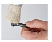
Lubricate the Snap-in valve with soap water or a mounting paste to decrease the friction between valve and rim hole, avoiding the valves surface damage.
