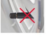
The valve stem should not extend out the rim flange.
