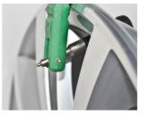
Use a suitable valve mounting tool. Do not stretch the valve to avoid damages. The pull-through of the valve has to take place in a straight line to the valve hole – do not tilt!
